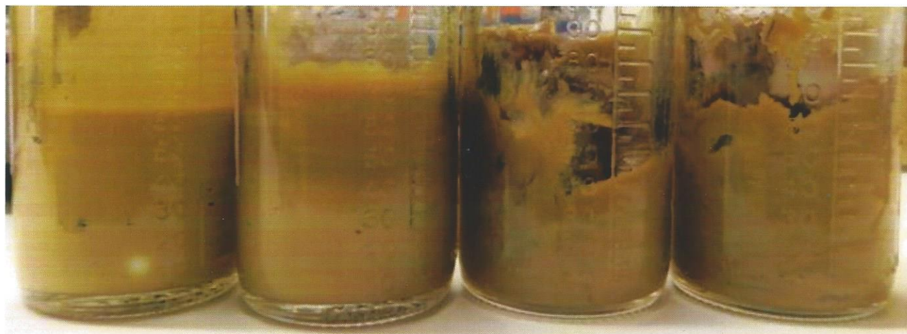
FIG. 5. Change in product consistency as water content is reduced from 80% to 30% (left to right) in an internal olefin sulfonate surfactant used for EOR.
